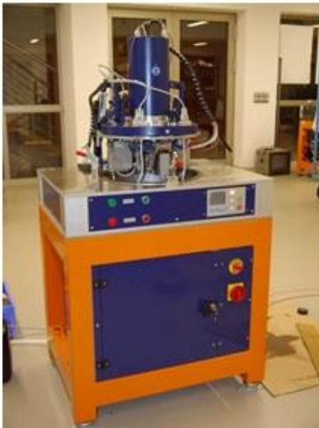
Piston Ring - Liner Simulator: Tetra GmbH
